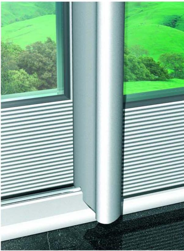
Thermal break system for sliding frames with inox steel roller driver and Hi-Fin bush sealing, based on a 38mm sash.
